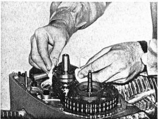
Insert camshaft into engine housing – push crankshaft sprocket on crankshaft carefully so that key and key groove mate. Install fixture sleeve, BMW tool No. 216, and puller bolt, BMW tool No. 535, over sprocket into the end of the cranshaft and pull the sprocket on. Caution – guide camshaft into its rear bearing bore.
