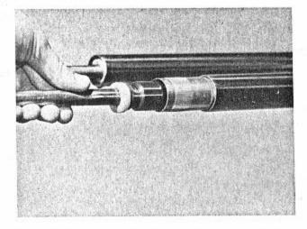
Remove springs from shock absorbers. Remove or install springs on shock absorbers by turning them to the right.
