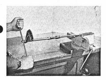
Assembly instructions: Reassemble shock absorber in reverse order. Clamp the hex, of the bottom retainer in vise and tighten both ends simultaneously by tightening at the hex. of the spring retainer. (for torque see 'Specifications').
