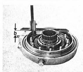
Adjust endplay to '0' without gasket. Use a depth gauge and a pair of prisms, BMW tool No. 50–36, and measure the distance from the ball bearing seat in the cover to the gasket mating surface of the cover (a).
