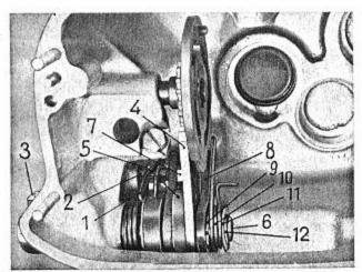
2) Insert the holders into the circular leaf spring and slide this assembly over the bushing, place the holders on each side of the short pin. Be sure that the crank of the levers is to the right (toward the selector).
