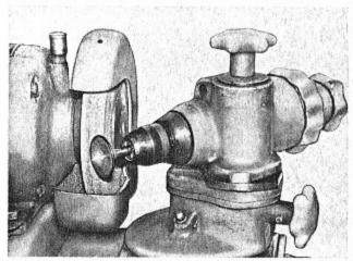
If necessary lap in valves using holder, pMvv 1001 No. 540.
