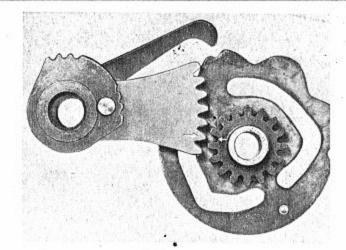
The over-shift ([a] between pawl and detent notches) is determined by the selector gear limiting bolts. The over-shift should be 1 mm (0.04") in 4th gear on the upshift and on 1st gear on the downshift. If necessary correct this by shimming. limiting bolts.
