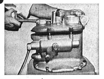
To install cover, heat it to 180 to 210° F. Place it on the transmission and depress kick starter partially. Move the kick starter up and down slightly to engage kick starter gear.
