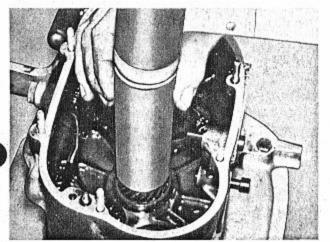
Place the divided plate p under the 1st speed gear (17), install the split plate upon an suitable press cylinder (c). Press off the speed gear together with thrust washer 19 and ball bearing 20.
