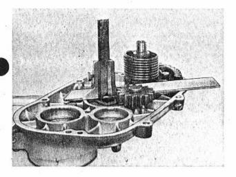
Measure from the mating surface of the transmission cover to the shoulder of the bushing installed in the bearing. The result has to be subtracted from the measurement obtained at the housing allowing for 0,1 mm (0.004") end play. The remainder has to be made up by spacers. b — (a-20) = 0,1 mm (b-[a-0.8"] = 0.004") = thickness of spacers required.
