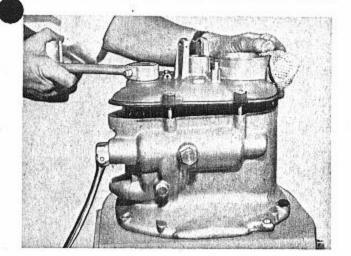
Check with inspection mirror and make certain that the the dewels are fully engaged into the sliding couplings, but that sliding couplings are not pressed against the gears.
