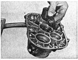
Remove bushing with shoulder from bearing. The determined cup shaped spacer (s) has to be placed on the bearing with the raised outer edge facing into the transmission. Reinstall bushing. The shoulder of the bushing must be included when measuring. We did so by installing it into the bearing before measuring.
